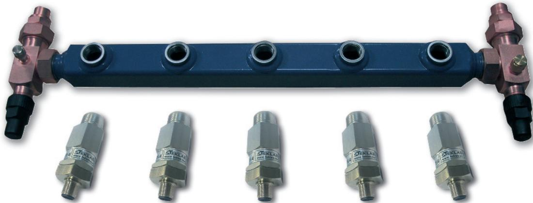
Teklab's STICK (Safe Tank Indicator Control Kit) is suitable where visual indication and/or control of the level inside a tank/vessel is needed. The unit comprises electro-optic sensors which have bodies made of stainless steel and dome made of glass: having no moving parts the reliability of the control is very high (SAFE). The units are customizable selecting the number of levels and the positions where the levels will be mounted.
